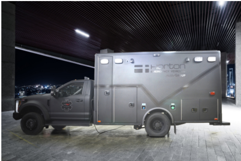
The REV Guardian, an ambulance wrapped in Level IIIA ballistic protection with run flat tire inserts (Photo: Business Wire)
