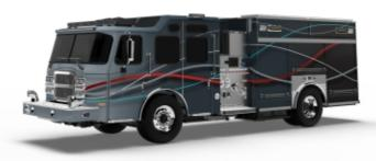
Mesa Fire and Medical Department purchases an E-ONE Vector, North America's First Fully Electric Fire Truck. The customizable Vector has the industry's longest electric pumping duration which allows four hose lines to be in use for four hours on a single charge. Additional features include a superior battery storage solution offering a safer, lower center of gravity and regenerative braking. (Photo: Business Wire)
